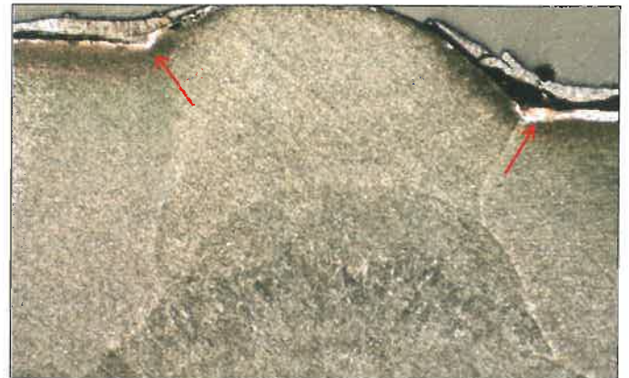
Figure 7. Copper fused into the surface layer of metal
