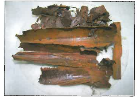
Figure 5. Flaky, copper deposits after chemical cleaning.
